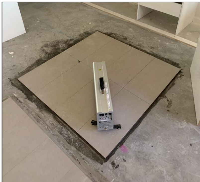
Figure 2. Source room & test 2 floor sample
