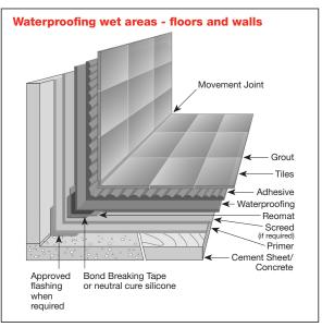
These diagrams are a guide only and should not be considered to be detailed designs. Final designs must be in accordance with AS3740:2021 and any applicable building standards.
